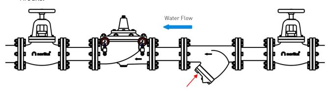
Note: A strainer must be installed before the pressure reducing valve to prevent damage from debris.
